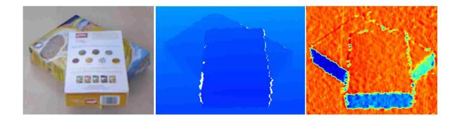
Figure 4.1: (a) RGB image of the scene,  $I_c$  (b) Color map of the raw depth map. (c) Color map of computed gradient direction image,  $I_{\theta}$
